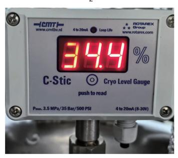
Reliable capacitive digital level gauge, decades using experience, enables our LN2 generator auto running and auto stand by.
